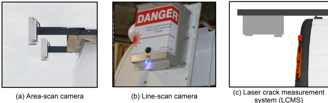
Figure 2 - Camera technologies for pavement surveys
