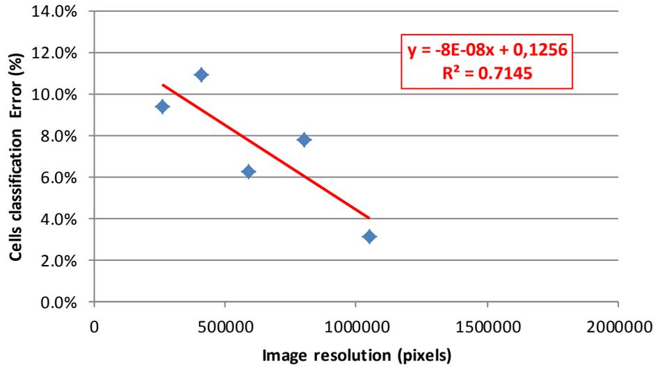
Figure 11 - Classification error according to the image resolution
